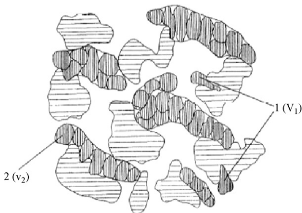
Fig. 13. Schematic representation of the anode structure (From ref. [55]).
